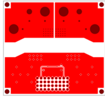
Figure 7. Board layout for measuring thermal resistance of CZ-3701
