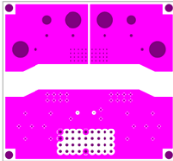
Figure 7. Board layout for measuring thermal resistance of CZ-3725
