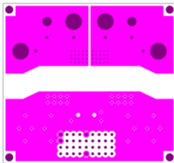
Figure 8. Board layout for measuring thermal resistance of CZ-3A02
