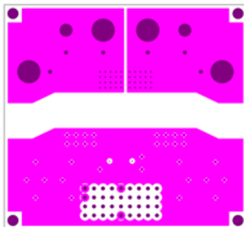
Figure 8. Board layout for measuring thermal resistance of CZ-3A04
