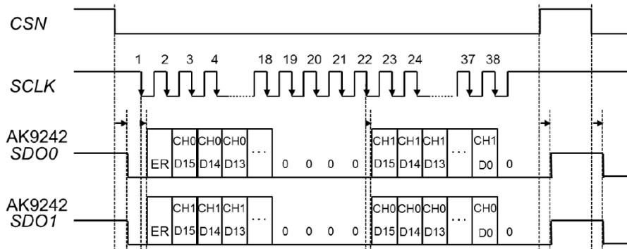
Figure 5. Data Output Timing in Serial Output Mode
