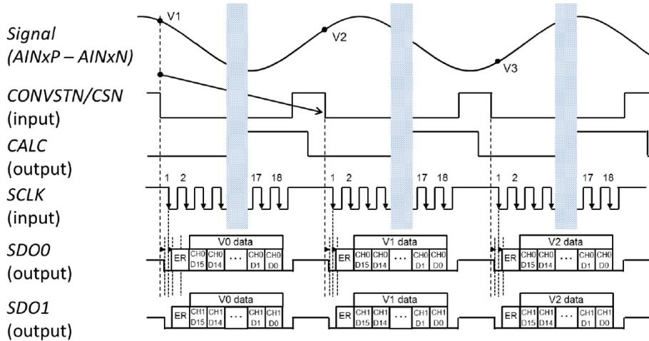
Figure 3. Data Output Timing (CONVSTN, CSN Common)
