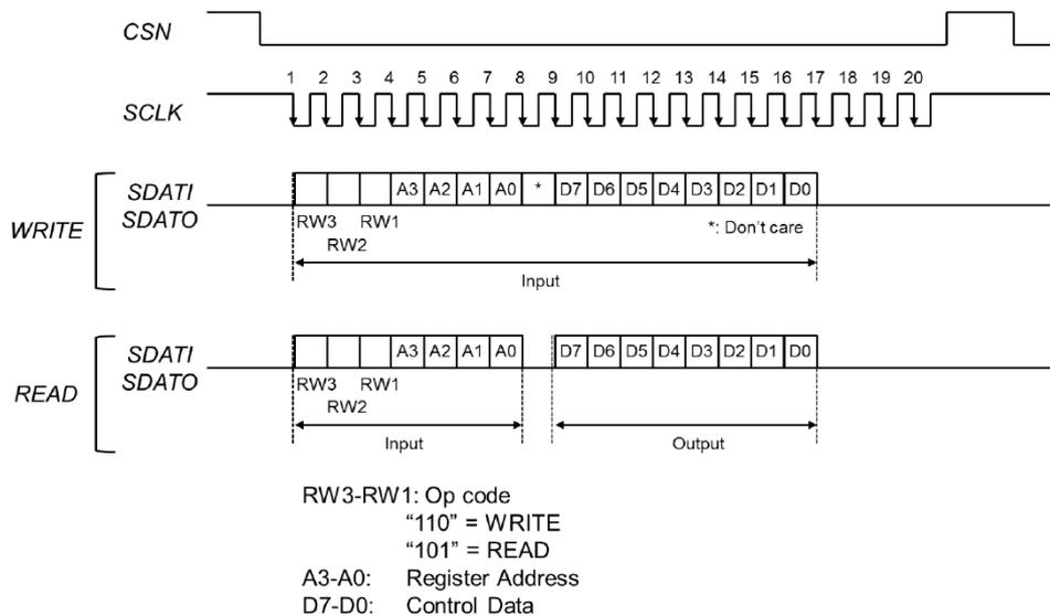
Figure 4. Serial I/F Timing (SDATI, SDATO Common)
